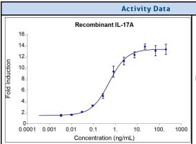
Recombinant human IL-17A (HZ-1113) stimulates dosedependent induction of alkaline phosphatase production in a HEK293 reporter cell line. Alkaline phosphatase production was assessed using pNPP as a chromogenic substrate. The EC50 was determined using a 4-parameter non-linear regression model. The EC50 value range is 0.24-1.2 ng/mL.
